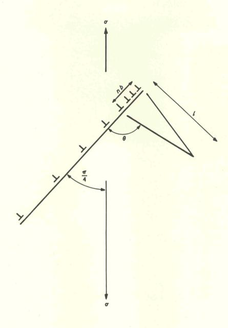
FIG I THE FORMATION OF A CRACK
